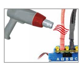
2. Slide heat shrink tube into the wires.
