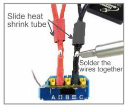
3. Slide heat shrink tube to exposed position and using heat gun or lighter to shrink it.
