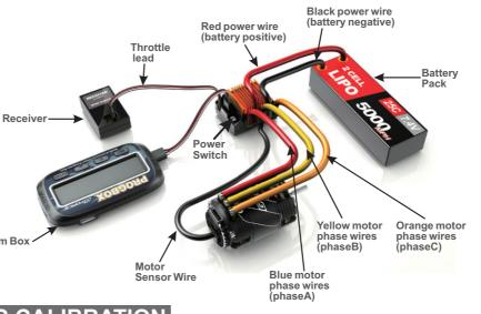
Choose a location for the speed control that is protected from debris. To prevent radio **Program Box** interference, place the speed control as far away from the radio receiver as possible and keep the power wires as short as possible. Select a location that has good airflow
